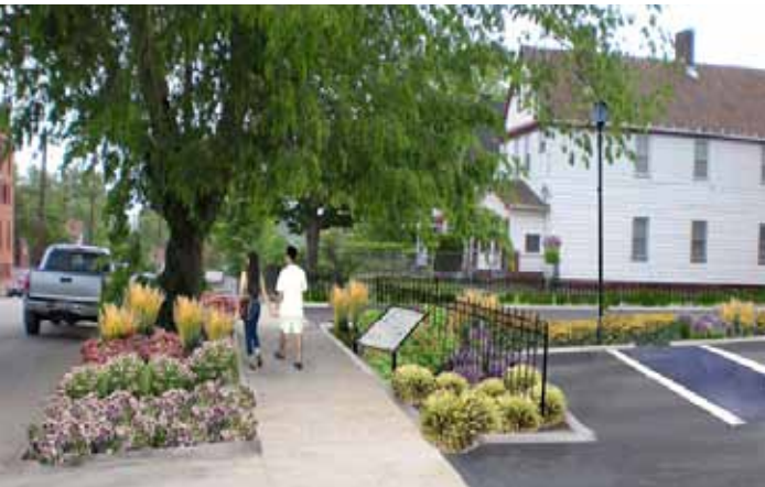
Illustration of a parking lot in Tremont neighborhood designed to provide bio-retention areas for managing stormwater
